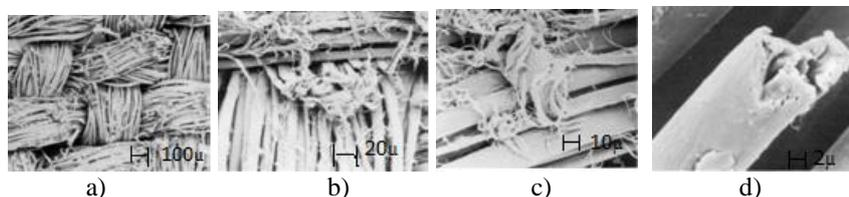
Fig. 5: Wear damage in silk dress after 60 years [13]
